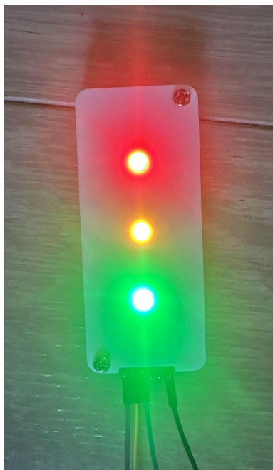
Figure 7 Exterior view of case with protoboard and all LED illuminated
