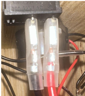
Figure 7 - Rocker switch Terminal Crimps
